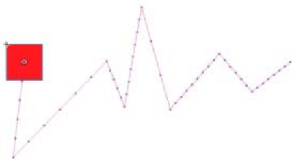
A motion path with roving keyframes turned off. Note the uneven distribution of frames, resulting in uneven speed of motion.
